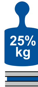
Horizontally mounted = 25% quoted load rating
