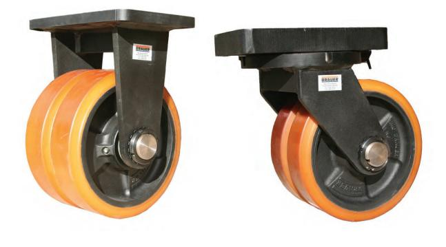
Wheel options of Cast Iron, Steel or Aluminium Vulkollan superior polyurethane is used as the standard tyre material.Tyres can be produced with crown/dome treads to suit specific applications. Bore options available for all standard wheels fitted with precision bearings. Operating temperature range -20C° to +60C°. Hardness of tyre of 92 ±3° shore 'A'.
