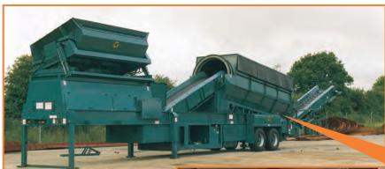
Drum supported on four pivoting castors each fitted with two polyurethane tyred wheels H200/60.
