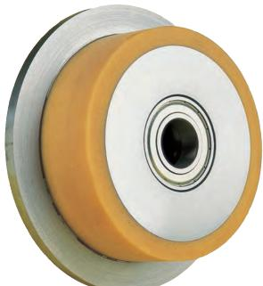
Standard wheel features flanges with a 5° angle and a 'flat tread' (ie tread parallel to the wheel axis) for running on flat top rail. Polyurethane is resilient, durable material, resistant to abrasion and to many common chemicals. Polyurethane tyred wheels are capable of carrying heavy loads and of transmitting driving forces.
