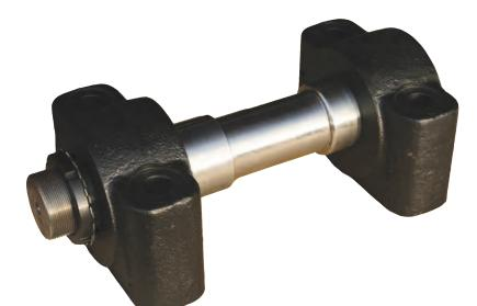
The 'BA' series axle assemblies are for mounting single wheels fitted with ball or roller bearings, the lock nut, lock washer, or self locking nuts and sleeve providing adjustment for opposed taper roller bearings.
