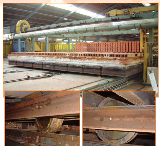
Wheels and axles supplied for the maintenace of dryer transfer cars for brick manufacturing plant. Brauer supplied complete wheel and axle assemblies that comprised Steel Double Flanged and Steel Flat Tread Wheels.
