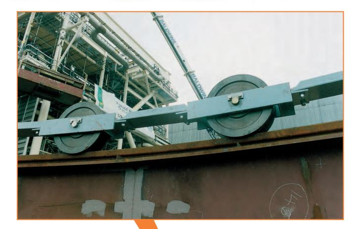
7600 tonne, 32 meter diameter, pipe laying turntable running on 330 steel double flange rail wheels fitted with self-lubricating bushes and stainless steel shafts. Tread diameter 450mm. Tread width 112mm wide with crown profile to assist tracking.
