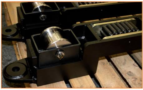
Brauer Ltd manufactured according to the design specification of J Murphy and Sons Limited, Gas pipe tunnel trollies for the gas ring main improvement to the west of London from Harefield to Southall for the National Grid.
