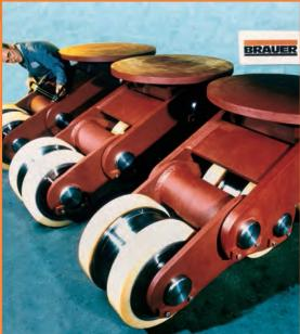
Wheel and axle assemblies used in a rotating drum application. Given the extreme conditions and high loadings involved the wheels and axles have been specifically designed to the customers requirements that demand flat tread wheels with axles that are capable of taking a load in excess of 75 tonnes.
