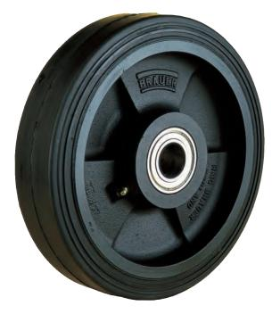
Rubber tyred wheels are the least expensive type of tyred wheel and are suitable for moderate loads. They are quiet in operation and protect the surface on which they run, although they can cause marking. Rubber tyres can generate static electricity, and where this is undesirable, 'anti-static' tyres can be specified.
