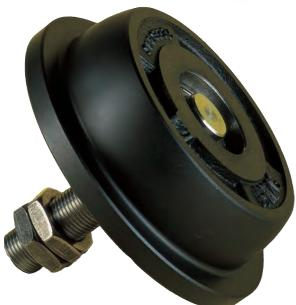
The SFR (cast iron) and SSFR (Steel) ranges of wheel assemblies have been designed to fit within standard sections of channel and 'l' beams. The radiused tread accommodates the angle of the section and improves the wear and tracking characteristics.
