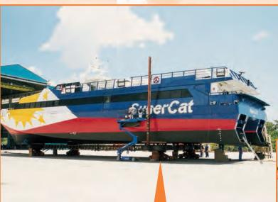
Multi-pivoting, dual purpose castor with directional swivel top plate. Fitted with 4 steel double flange rail wheels, 450mm tread diameter and 90mm tread width and 8 anti-hydrolysis polyurethane tyred wheels, 505mm tread diameter and 150mm tread width. All axles are ground stainless steel running in self lubricating nylon bushes.
