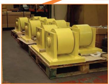
This ship mounted pipe laying turntable which is running on three rings of tapered tread steel wheels mounted in a fixed frame. The wheels and frame are finished in marine specification paint. Total weight when loaded is 600 tonnes with each wheel and bracket capable of carrying 50 tonnes.
