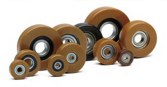
Temperature range of operation -40° to +85°C. The polyurethane is non-marking, with high resistance to axial loading, and runs quietly. Used in conveyor applications, systems of transporting products along material handling systems or in areas of support for hanging structures or components, as found in;
