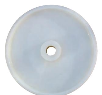
Plain untyred nylon wheels are the least expensive type of wheel. They are light in weight, and are resistant to impact, abrasion, corrosion, and the effect of many chemicals. They can be fitted with bearings but are most often used with their nylon bores running on a smooth steel axle. No lubrication is necessary, but they will benefit from being oiled. Having little resilience they tend to be noisiest when moving quickly over rough surfaces, and they can mark floors if highly loaded.
