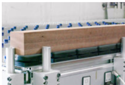
Innospann Steel-Plate mounted on a flat table
