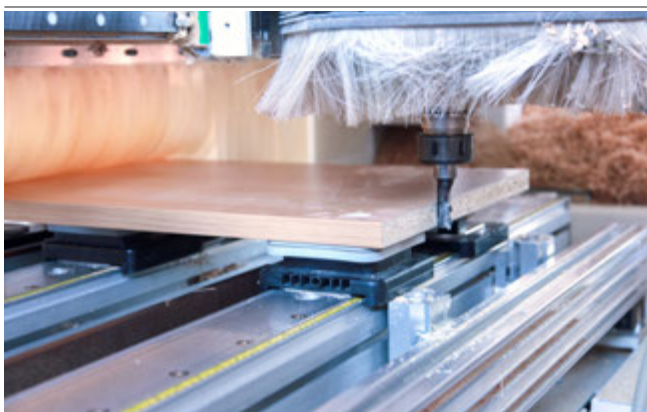
Vacuum block VCBL-S4 used with SCM consoles
