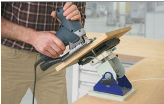
Multi-Clamp VC-M for manual processing of wooden workpieces
