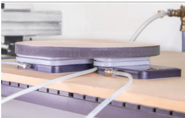
Vacuum Blocks VCBL-G-K1 for clamping MDF workpieces
