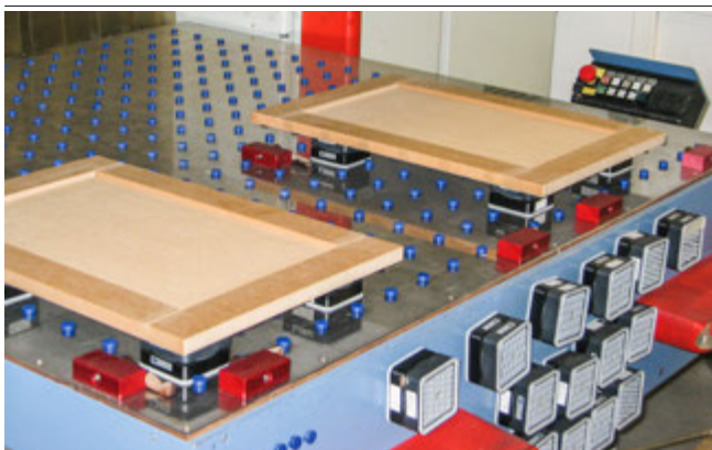
Innospann Steel-Plate with Mono-Base and suction cups
