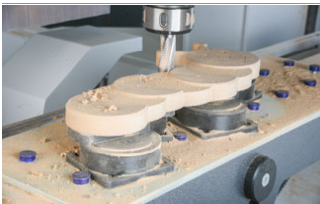
Adapter-Plates ISAP-K1 with Mono-Base and suction cups for clamping curved wooden parts
