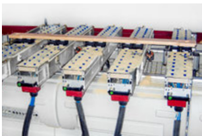
Innospann Steel-Plate mounted on a console table
