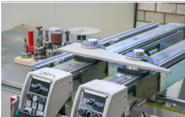
Mechanical Clamps VCMC-S4 for clamping wooden parts
