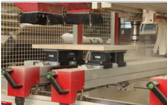
Vacuum Blocks VCBL-K2 while clamping a workpiece
