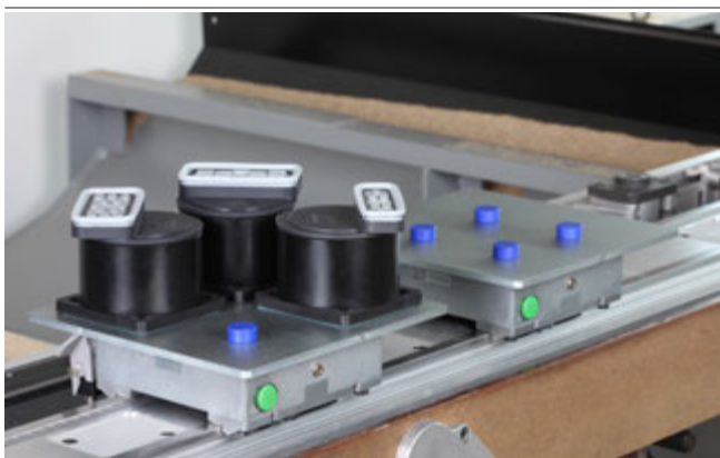
Adapter-Plates ISAP-B with Mono-Base and suction cups for clamping wooden components
