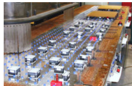
Innospann Steel-Plate mounted on a grid table
