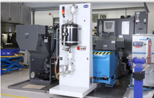
Vacuum Operation Center VOC for vacuum generation in wet working conditions
