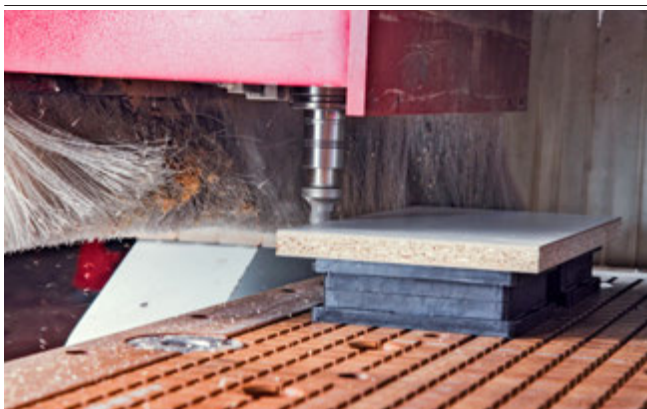
Vacuum blocks VCBL-R for gripping particle boards
